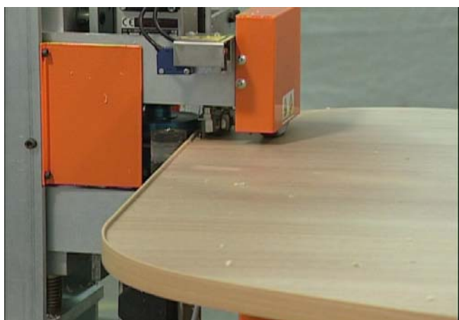
Second phase: Trimming of the edge
