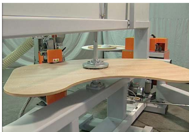
Second phase: Trimming of the edge
